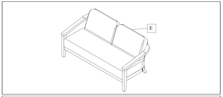
Place Back Cushions (E) onto the assembly as shown. **Note**: that the Back Cushions (E) are directional and should be oriented correctly. The Bench is now fully assembly and ready for use.
