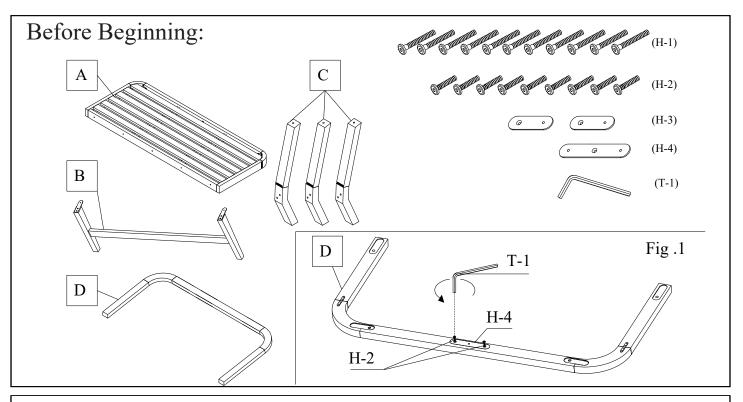
Please use Allen Key (T-1) to remove 2x Small Bolt (H-2) and Large Metal Bracket (H-4) attached on the Backrest before beginning assemble. See fig.1
