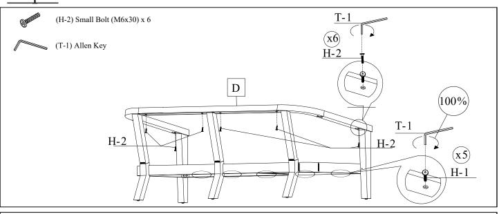
Position the Backrest (D) onto the assembly, ensuring the Large and Small Metal Brackets (H-3 and H-4) and the brackets on the Front Frame (B) nest into the mortises under the Backrest (D). Loosely secure with Small Bolts (H-2) using the provided Allen Key (T-1). Fully tighten ALL hardware from this and all previous steps at this time. DO NOT OVER TIGHTEN.
