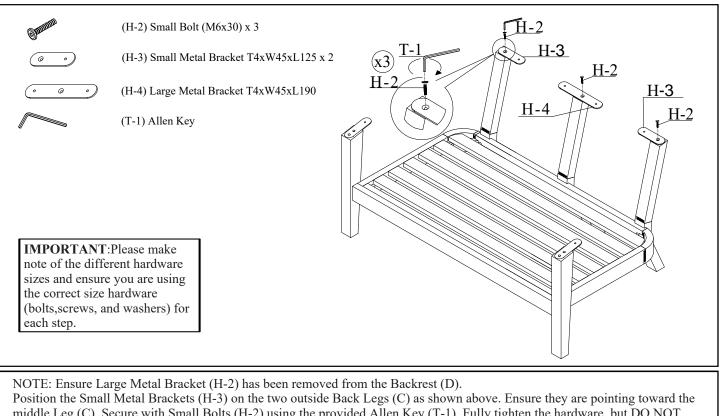
middle Leg (C). Secure with Small Bolts (H-2) using the provided Allen Key (T-1). Fully tighten the hardware, but DO NOT OVER TIGHTEN. Position the Large Metal Bracket (H-4) onto the middle Leg (C) and secure with a Small Bolt (H-2) using the provided Allen Key (T-1). It is important to FULLY TIGHTEN all hardware in this step at this time. DO NOT OVER TIGHTEN.
