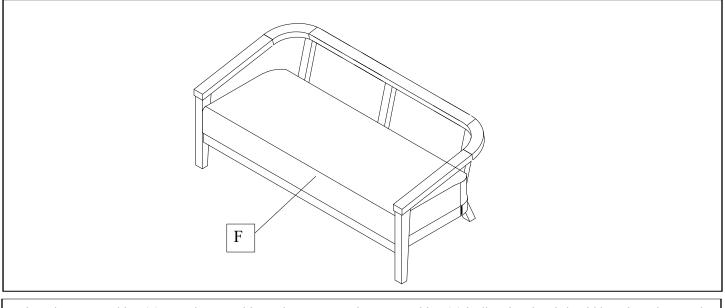
Place the Seat Cushion (F) onto the assembly as shown. Note: the Seat Cushion (F) is directional and should be oriented correctly.
