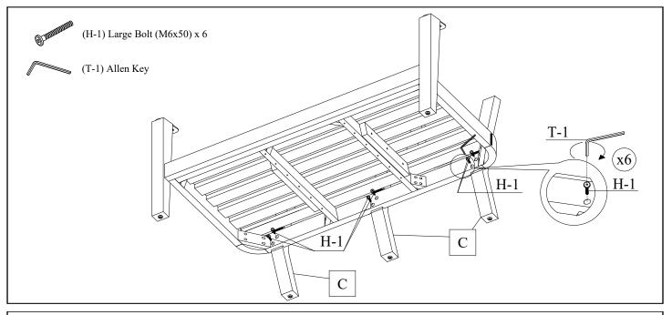
Position Legs (C) to the back of the assembly as shown above. Align the through holes in the Seat Frame (A) with the receiving holes in the Legs (C). Loosely secure with Large Bolts (H-1) using the provided Allen Key (T-1). Do not yet fully tighten.
