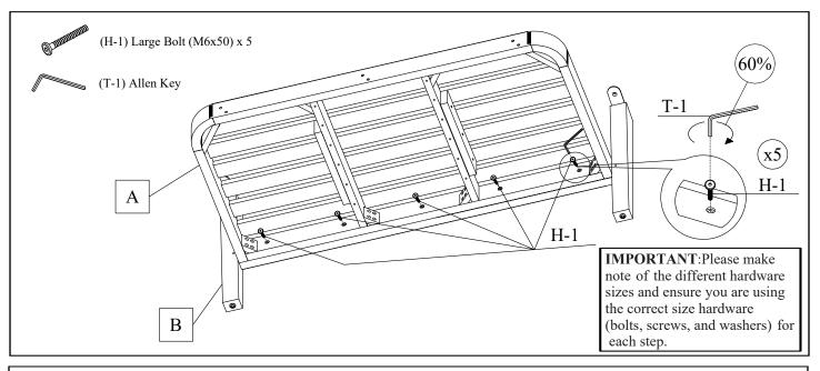
Using a second person to assist you, position the Front Frame (B) with the Seat Frame (A) as shown above. Align the through holes in the Seat Fame (A) with the receiving holes in the Front Frame (B). Loosely secure with Large Bolts (H-1) using the provided Allen Key (T-1). Do not yet fully tighten.
